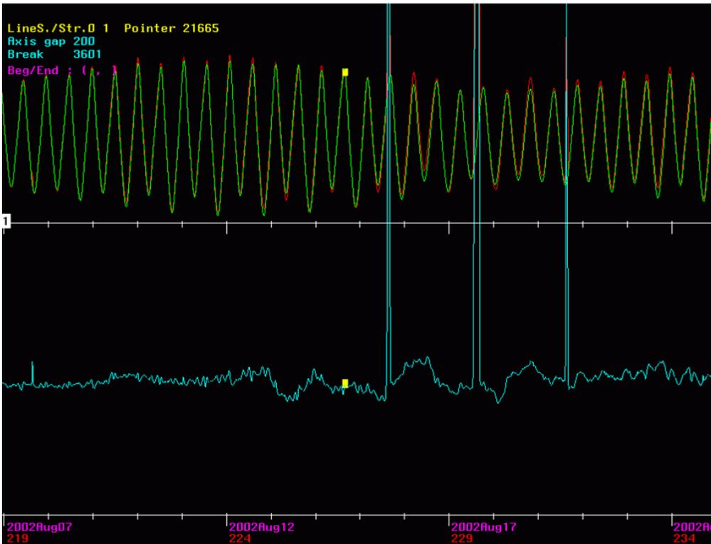
Figure 13 – Example of timing error caused by clock malfunction
