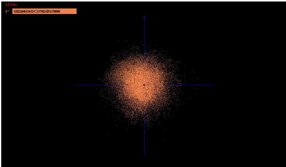
Figure 14 shows an example of a 'good' scatter plot. There seems to be an even array of wind directions indicating that the compass was not being hindered. However, Figure 15 below is an example of a record with suspect directions, as there are very few measurements between 80 and 100 degrees, or between 260 and 280 degrees.
