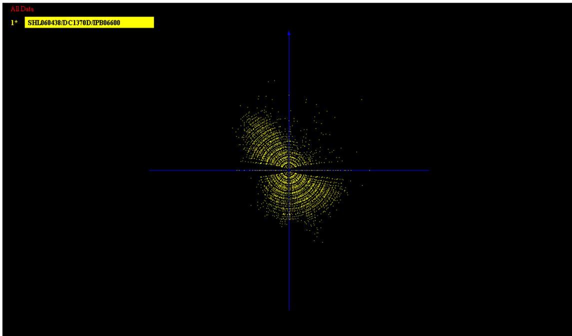
Figure 15 shows an example of a scatter plot that invites further investigation. In this instance, as a number of directions of 90 or 270 degrees were recorded, it was decided that there was no compass error, although possibly a shadowing effect of the placement of the anemometer.
