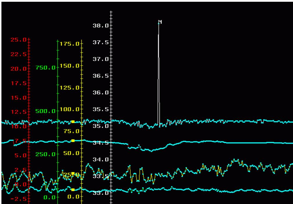
Figure 3 gives an example of a 'spike' in salinity within a series. The spike has been flagged as suspect with the customary 'M' flag. As can be seen only one point is out-of-range indicating it is likely to be an instrumental error.
