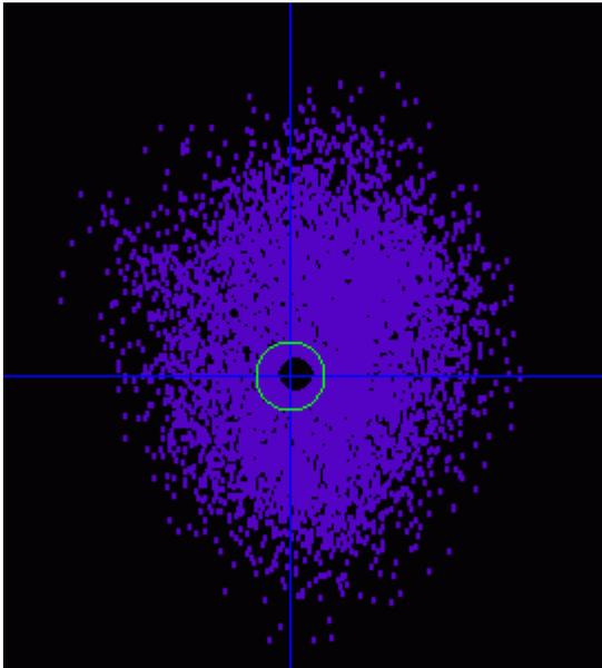
Figure 6 shows an example of a 'good' scatter plot. There seems to be an even array of current directions indicating that the compass was not being hindered.
